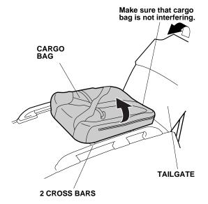
2. With the help from an assistant, carefully unfold the cargo bag on the cross bars.
