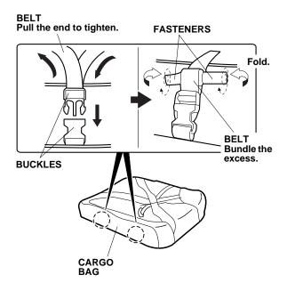
20. Bundle the excess belt ends on the buckles as shown and fold the fasteners inward to secure the belts on the buckles.
