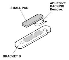
7. Remove the adhesive backing from the small pads and attach them to the brackets B.
