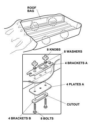
9. Loosely install a bracket A, a plate A, and a bracket B to the cargo bag with two bolts, two washers, and two knobs at each location shown. Be sure the cutout on bracket B is facing the outboard side of the vehicle. Make sure the pads on plate A and bracket B are facing each other. 10. With the help of an assistant, carefully place the cargo bag on the cross bars.
